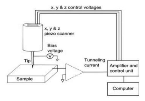
FIGURE 2: SIMPLIFIED SCHEMATIC OF A SCANNING TUNNELING MICROSCOPE (STM) [21]. **Types of Nanomaterials**
