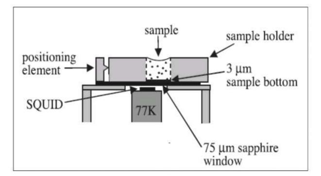
FIGURE 2: Simplified schematic of measurement of magnetic flux using squid (Ramane, 2020).
