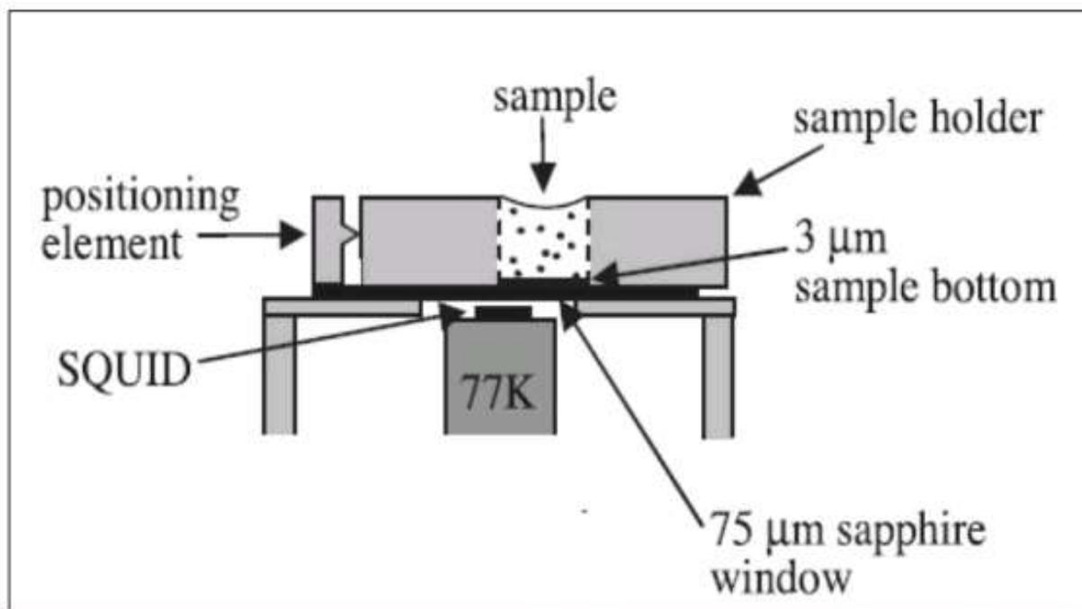
FIGURE 2: Simplified schematic of measurement of magnetic flux using squid (Ramane, 2020).
