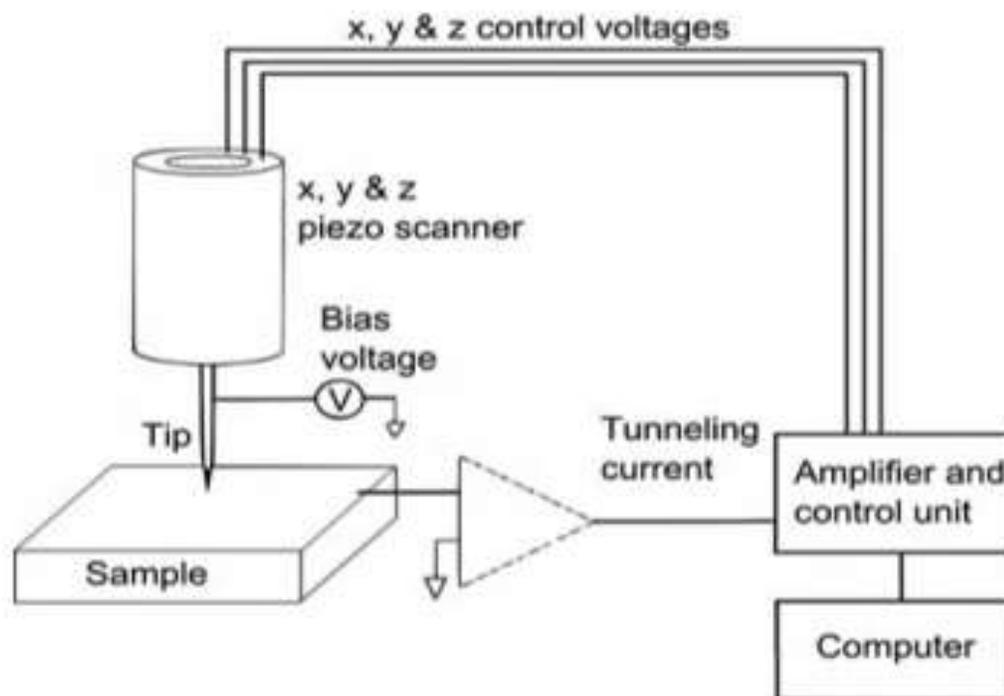
**FIGURE 2: SIMPLIFIED SCHEMATIC OF A SCANNING TUNNELING MICROSCOPE (STM) [21].**
