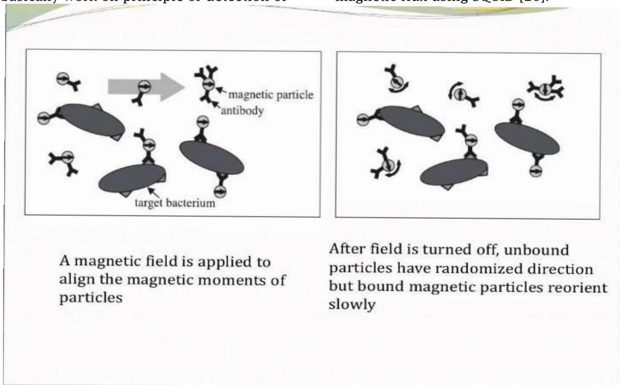
**FIGURE 4: Schematic showing alignments of magnetic particles [26].**
