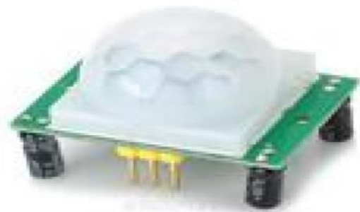
Figure 5: Passive Infrared (PIR) Sensor
