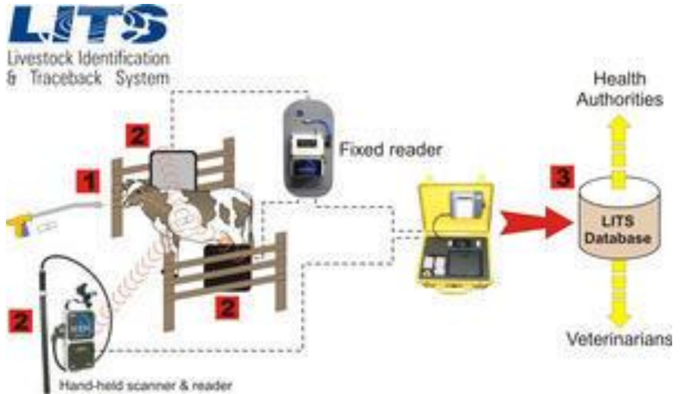
Figure 1: Application Architecture of Bolus Tracking System (BTS)
