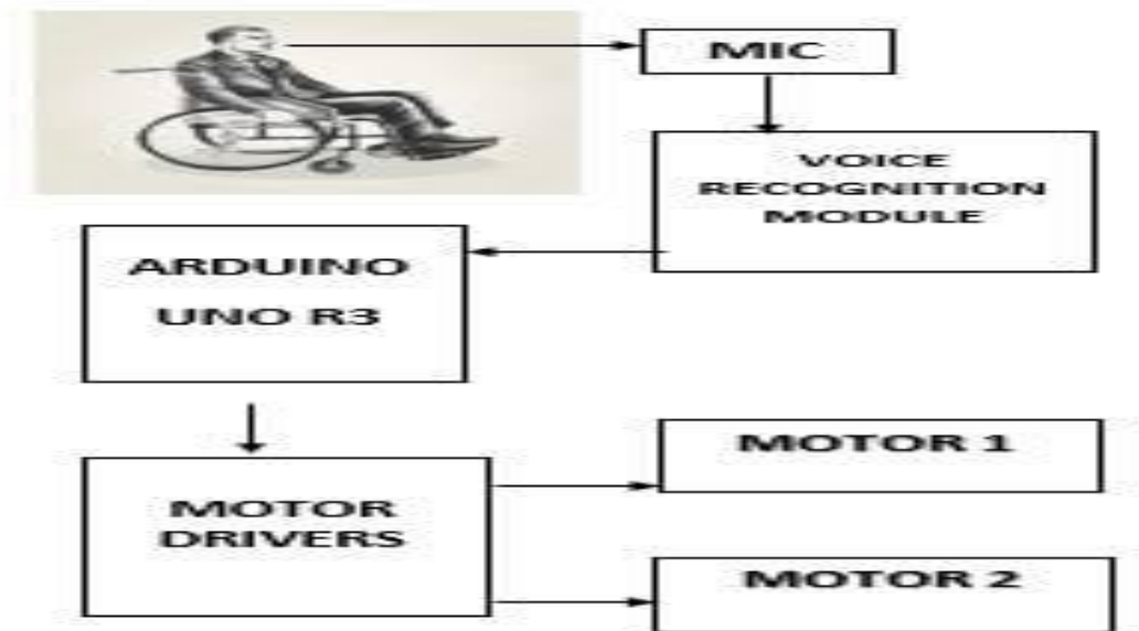
Figure 1: Showing the System Architecture
