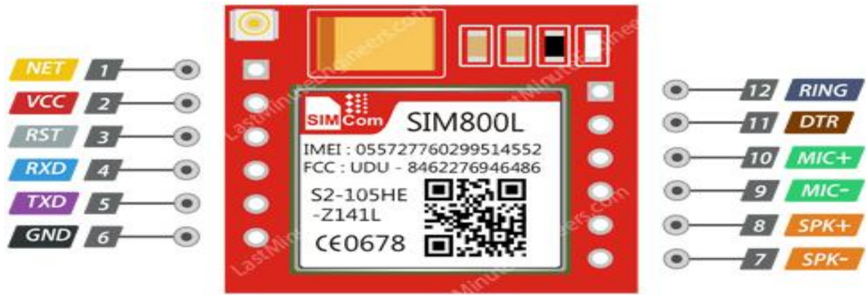
Figure 4: SIM800L GSM Module Pinout
