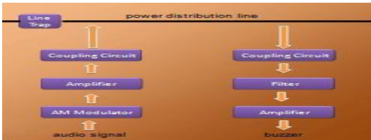
Figure 1: Block Diagram of PLC System Design.
