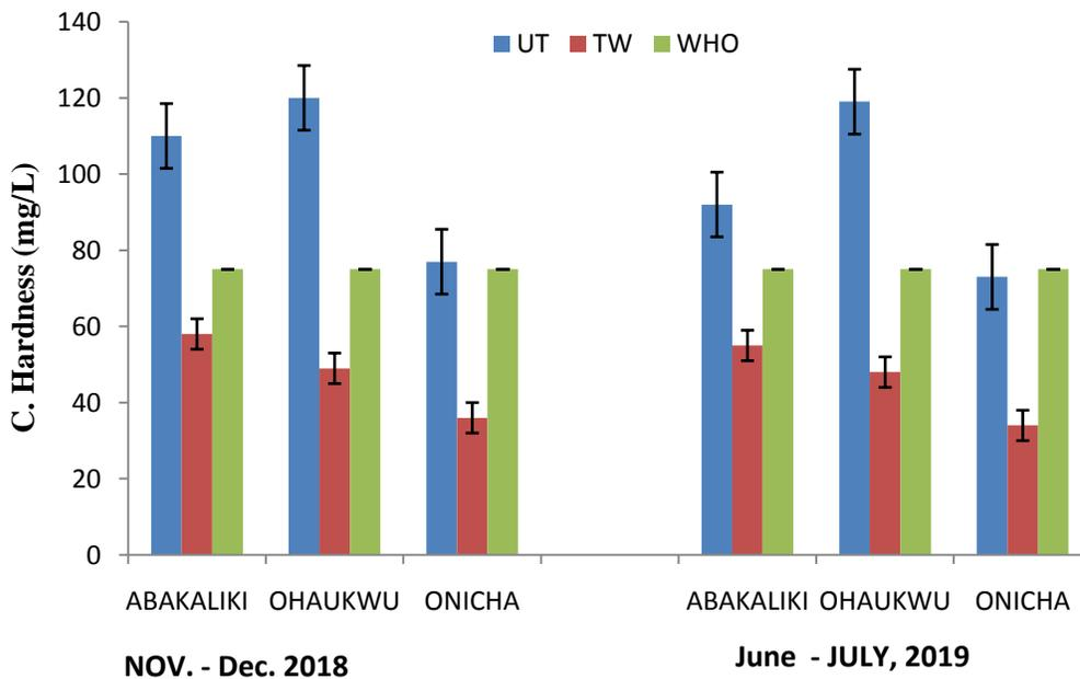
Fig. 2: calcium hardness concentration of the Borehole Samples (UT = untreated, TW = treated)
