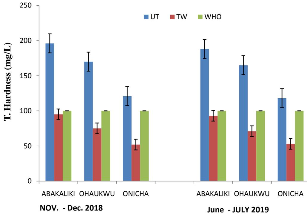
Fig. 1: Total Hardness concentration of the Borehole Samples (UT = untreated, TW = treated)
