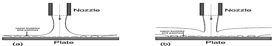
Fig. 1.: Schematic diagram of water impinging as a jet onto a surface (a) the free surface and (b) plunging jets.
