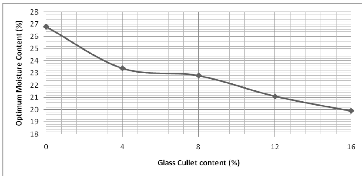
Figure 2 Variation of Optimum Moisture Content with Glass Cullet content
